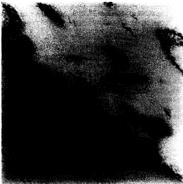
Figure 15 TEM photograph of the domain boundary between PA6 and PC in 25/75/5 PA6/PC/SEBS-gMA where SEBS-gMA is stained with RuO 4
