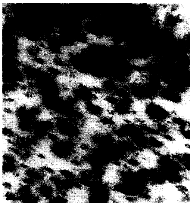
Figure 5 TEM photograph of 100/10 PA6/SEBS-gMA binary blend stained with RuO 4
